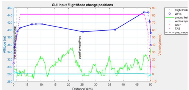
Figure 5. Flight mode input GUI in which the flight path is plotted above the ground height curve.
